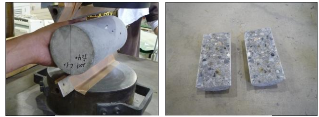
Fig.1 Method of splitting specimens
