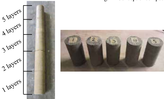
Phot.1 Appearance of 5 layers rammed earth wall specimen and rammed earth wall specimen after cutting
