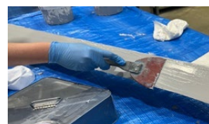
(c) Application of elastic putty
