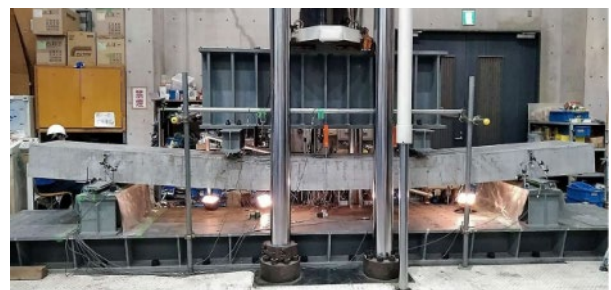
(a)At ultimate bending failure
