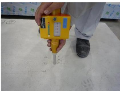
Fig. 4 Rebound hammer test
