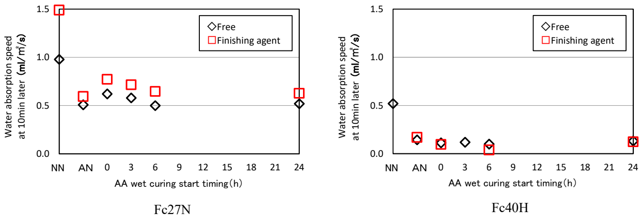
Fig. 4 Test results of water absorption
