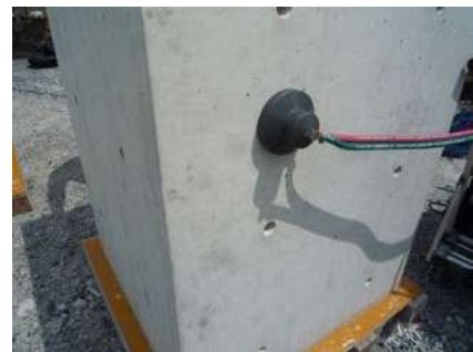
Fig. 5 Air permeability test
