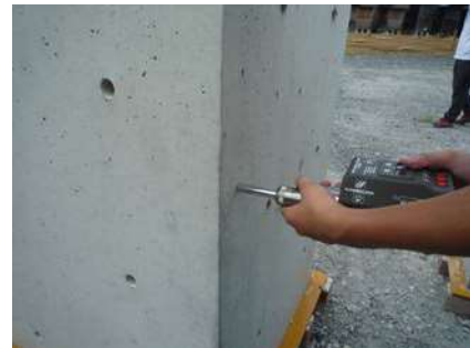
Fig. 6 Rebound number test
