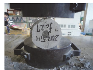
Fig.7 Tensile strength test
