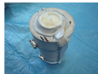
Fig.6 Removal of sealing material
