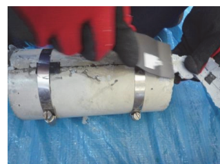
Fig.6 Removal of sealing material
