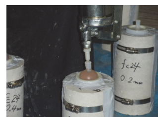
Fig.5 Injection of epoxy resin into concrete cracks
