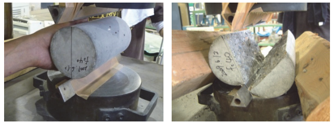
Fig.1 Method of splitting specimens
