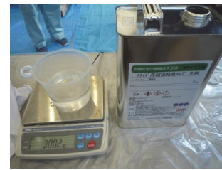
Fig.4 Preparation of ultralow viscosity epoxy resin
