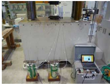
Fig.8 Water absorption test
