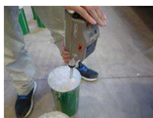
Fig.5 Rebound hammer test
