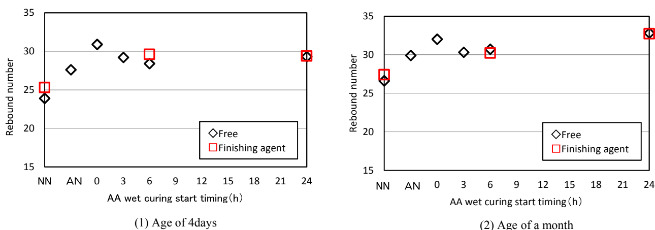
Fig.11 Effects of curing methods on rebound number
