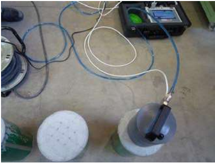
Fig.7 Air permeability test
