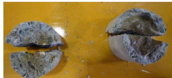
Discolored boundary by chloride ions
