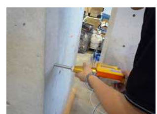
Fig. 6 Rebound number test
