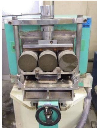
Photo2 Grinding of specimens (Left : \phi 100 Right : \phi 75 )
