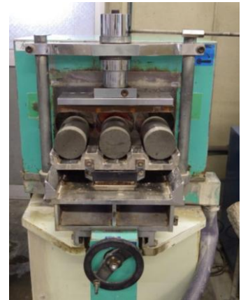
Photo2 Grinding of specimens (Left : \phi 100 Right : \phi 75 )
