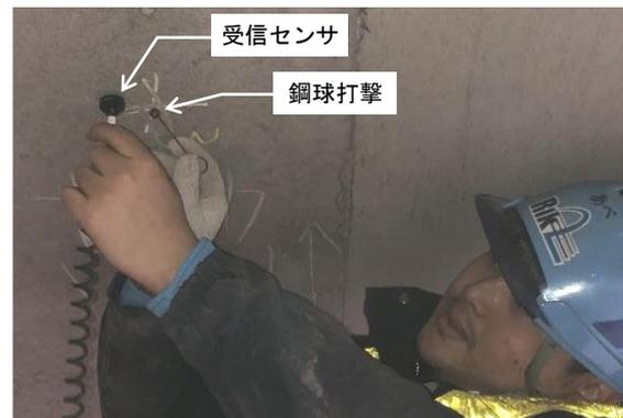
Fig.6 Measurement situation of Impact Elastic Wave Method
