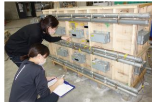
(g)封緘養生温度測定
