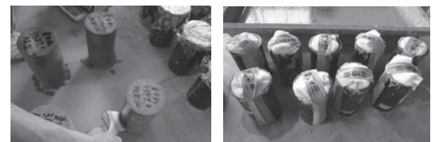
Membrane curing Wet curing
